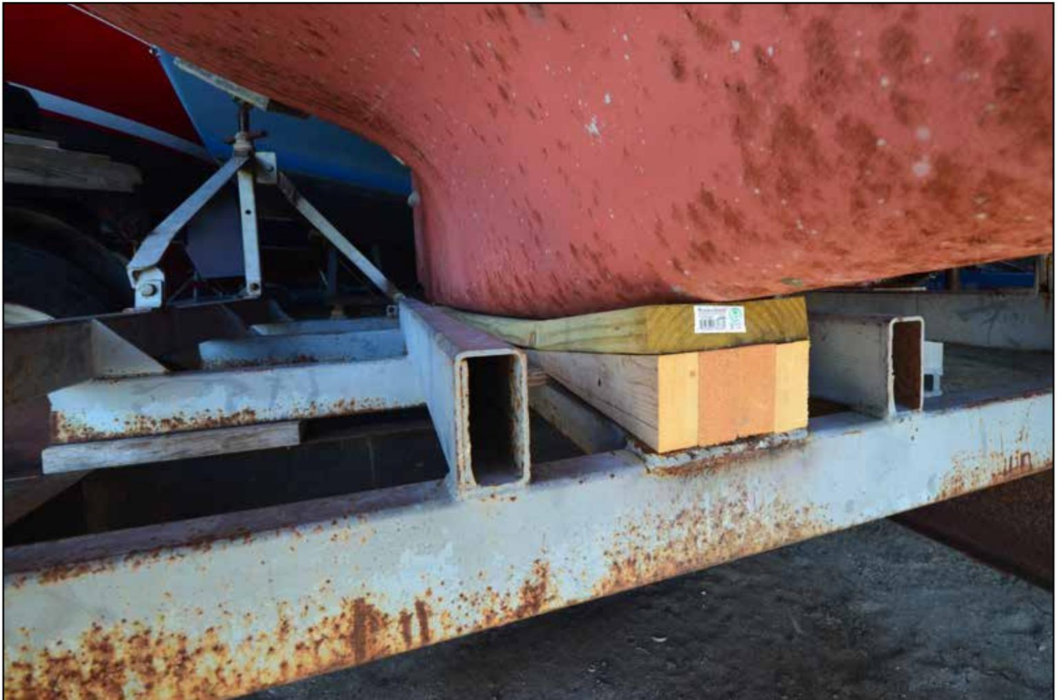
The wood keel support angles to accommodate the shape of the Flicka keel.
