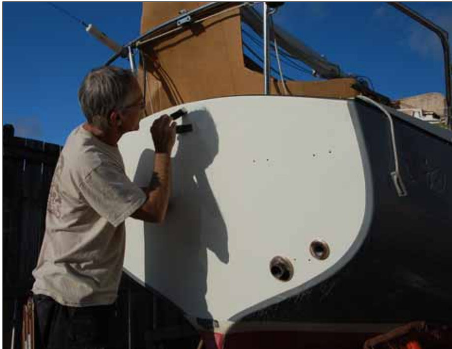
Matching the original gelcoat would be difficult due to fading of the gray gelcoat, so the transom was painted white.
