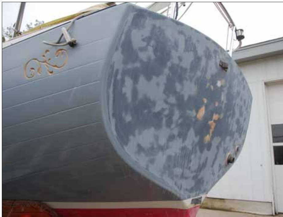
After the West System repair was completed, the transom was brought back to the original shape.
