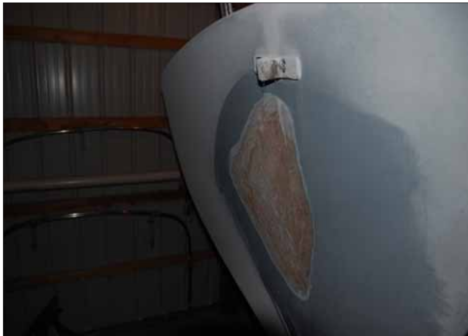
Sanding was required to remove the gelcoat separated from the fiberglass on the transom of BEN MAIN, Jr.
