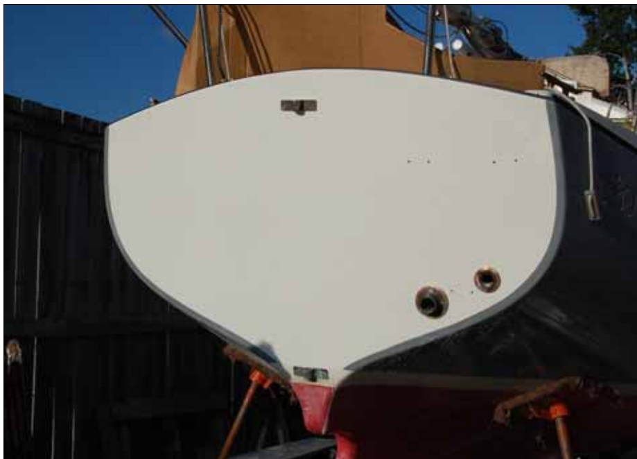
The gray gelcoat along the edge of the transom was not sanded or painted, giving the appearance of wood planking.
