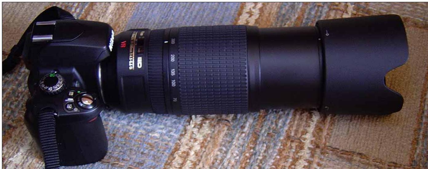
The Nikon 70-300 mm zoom was selected for my telephoto lens. It is equal to a 105 to 450 mm zoom on a full frame 35 mm camera.
