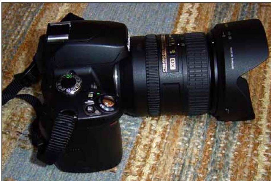
**The Nikkor 16-85 mm Lens is used most of the time. It is equal to a 24 to 127.5 mm lens on a full frame 35 mm camera.**
