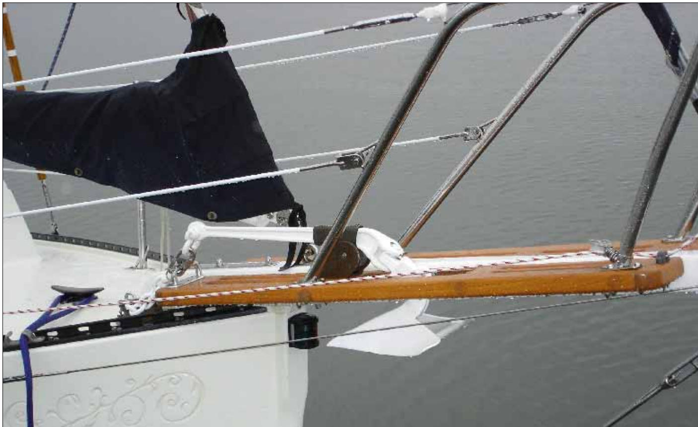
While this bowsprit appears to be a factory bowsprit, the central white portion is aluminum. Photo: Steve Grisanti © 2006
