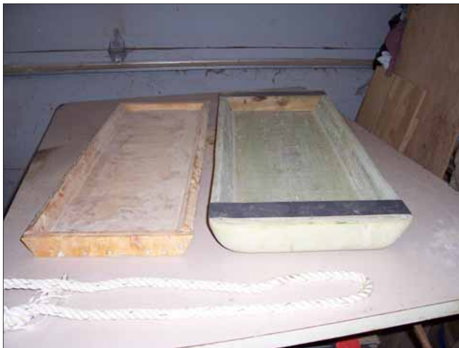
Shutters are being constructed to cover the two large aft ports.
