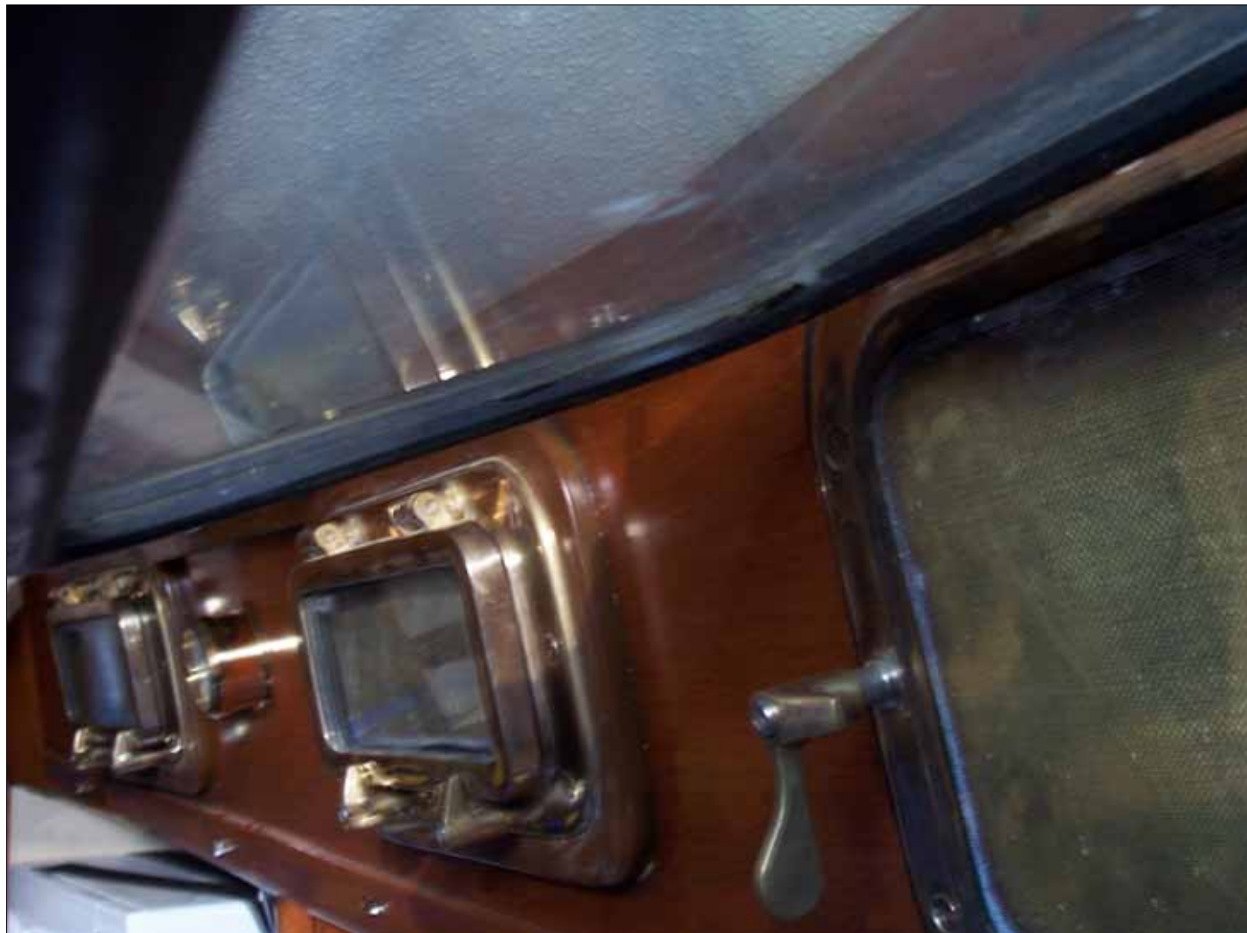
Two large ports were used aft. Note the insect screen in the large port and the teak spacers for the two smaller ports located forward.
