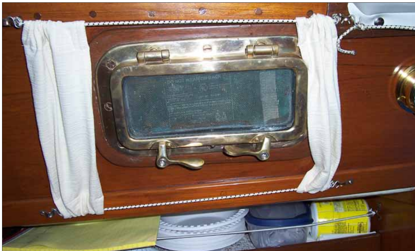
Two large ports were used aft. Note the insect screen in the large port and the teak spacers for the two smaller ports located forward.
