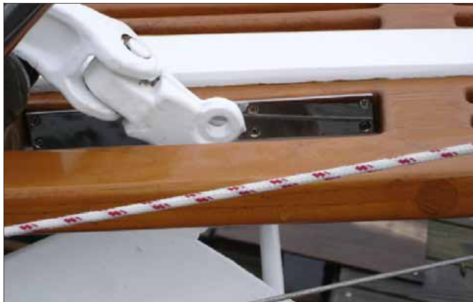
Stainless steel plates were added to protect the teak from the anchor. Photo: Steve Grisanti © 2006
