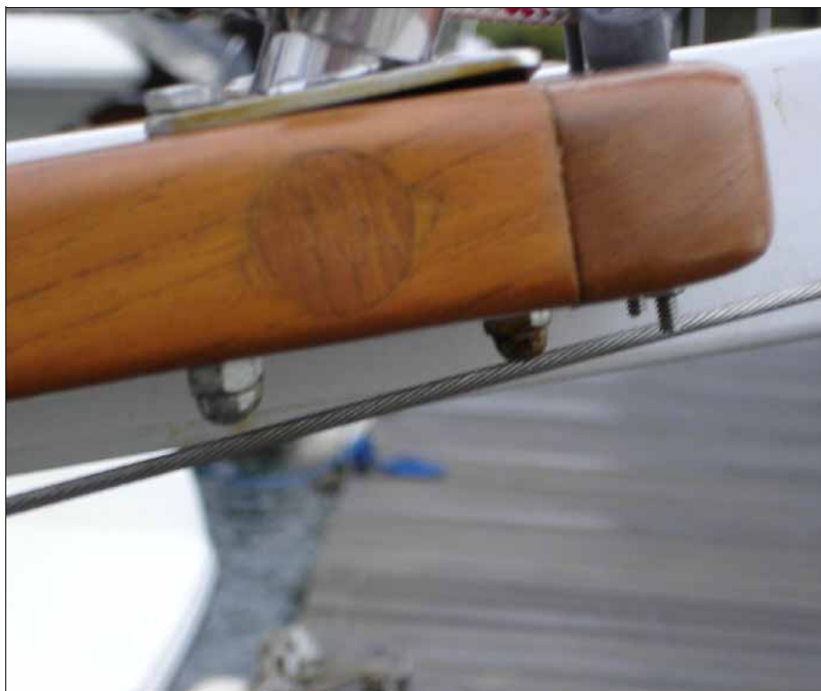
The platform holes were sealed using with teak plugs. Photo: Steve Grisanti © 2006
