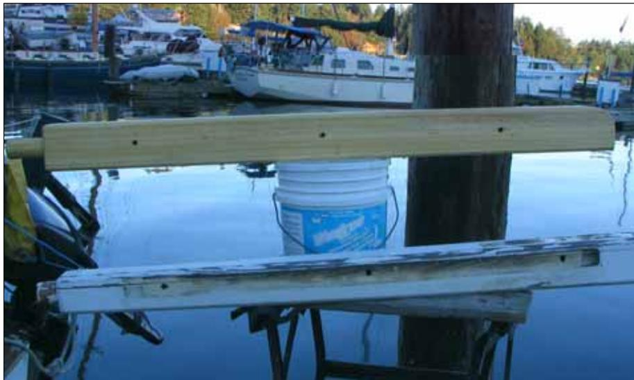
**Here is the old bow sprit and the new replacement. The new one has a larger cross-section than the factory original allowing the platform holes to be drilled closer to center.**
