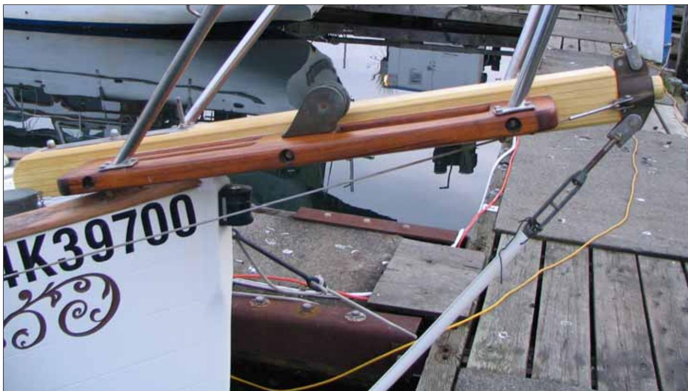
The first bolt will be used to secure the staysail.
