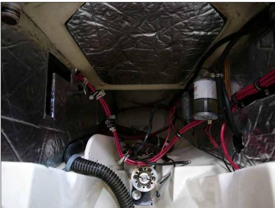
A layer of sound proofing was also added to the engine hatch. Also, notice the new gel coat finish in the engine bed.
