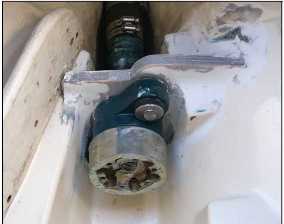
**After considerable trial and error, the thrust fitting was installed.**
