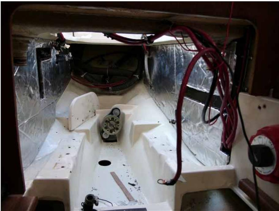
With the engine out, sound proofing was added to the engine compartment.
