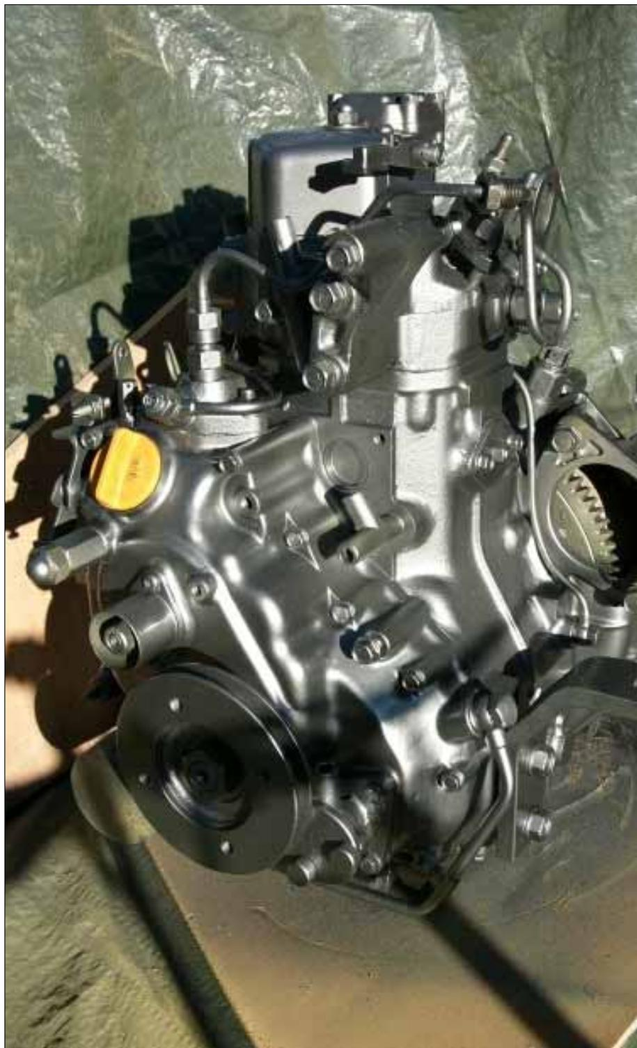
The Yanmar looks much better after cleaning, priming and a fresh coat of factory paint.
