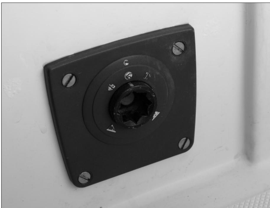
Unlike the original two lever arrangement, the Spinlock lever can be removed when not needed. This prevents mainsheet complications.
