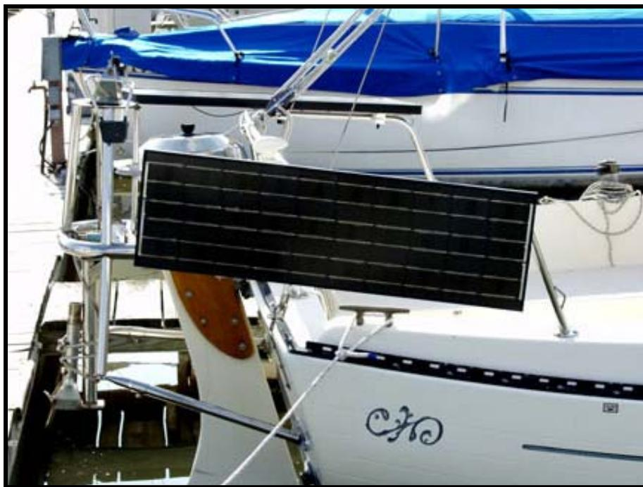
The solar panels are attached to the stern pulpit.
