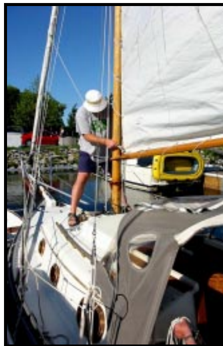
The lacing tension is adjusted to allow the gaff to move to the top of the mast.
