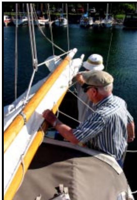
This line is laced fairly tight. Unlike on the mast, there will be little sail movement.
