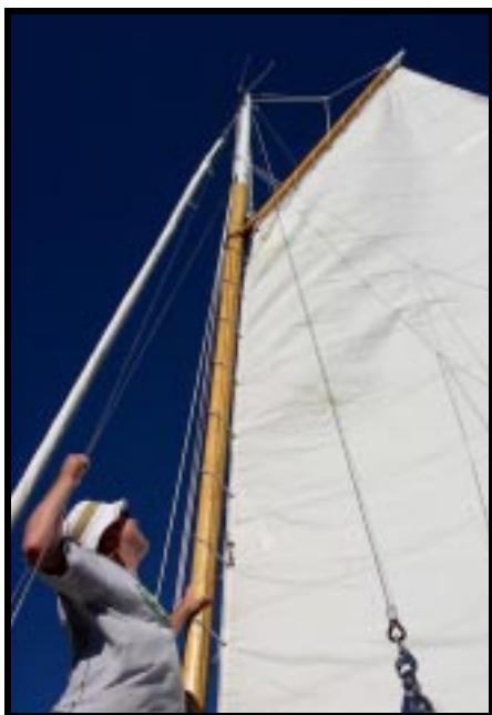
Once the gaff is at the top of the mast, the lacing can be correctly adjusted and secured.
