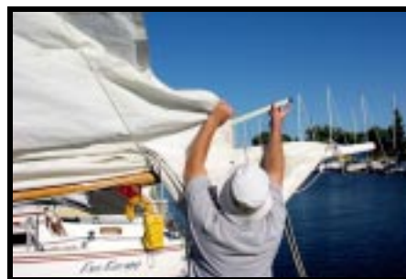
The lacing tension is adjusted to allow the gaff to move to the top of the mast.
