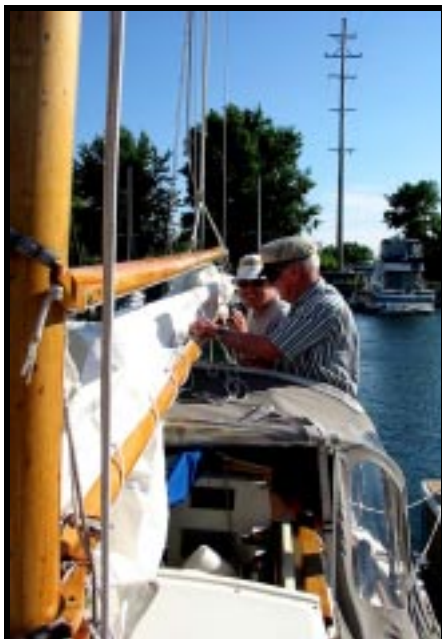
The mainsail is laced forward to aft using three-eighths inch twisted rope.
