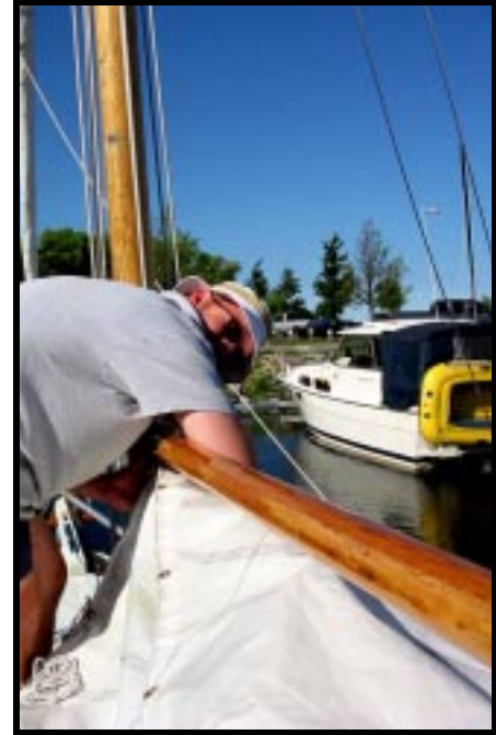
The sail is secured to the forward end of the boom. Next, the out-haul is attached at the aft end.
