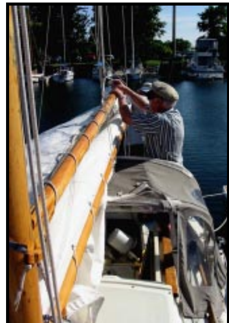
The same lacing process is repeated on the gaff. Like the line on the boom, it is laced tight and secured.
