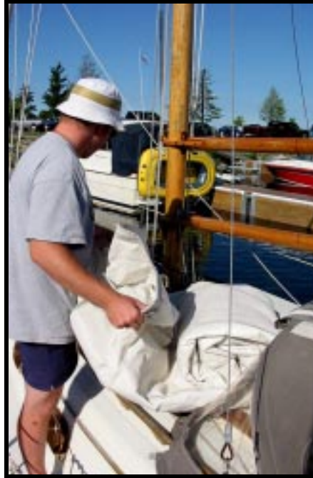
Dick's son unfolds the mainsail and prepares it for lacing to the boom, gaff and mast.
