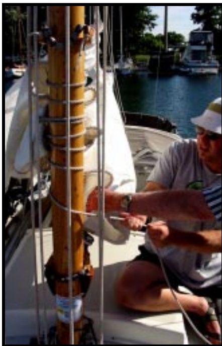
Initially fairly tight to thread the grommets, the mast lacing will be loosened as the sail is
