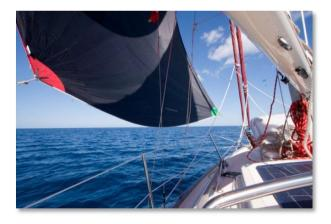
Caraway has a black asymmetric spinnaker made by Momentum Sails. It's the type B which means it is the fuller cut of their two standard shapes. You can't go so close in it but it is better off the wind.
