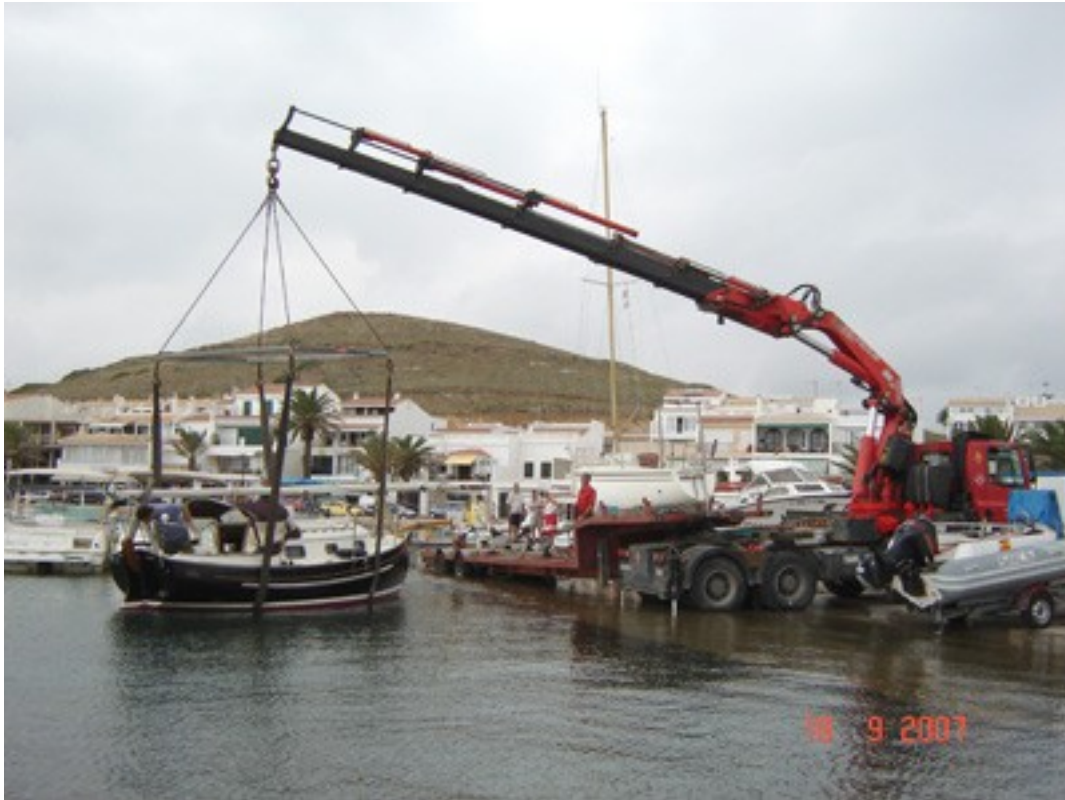
Small boats such as the Flicka can be launched with a mobile crane. Try that with a 40 footer!
